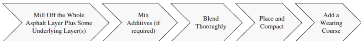
Figure 20 Basic steps of full-depth reclamation (FDR)
